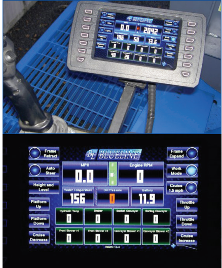
Modern controls with touch screen and digital readouts
